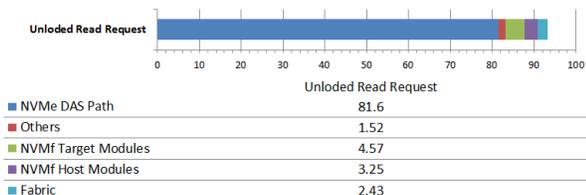
Figure 8: A breakdown of NVMe end-to-end latency for an unloaded read request.
